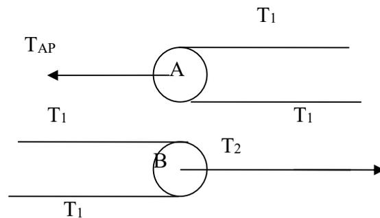
$$T'_1 = T_1 = T'_{A2} = T_{A2} = T_{A3} = T_1 \quad (15)$$
